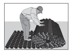
**Specifications:** EZ Roll™ Grass Pavers are honeycombed rolled grass paver that are comprised of 24" x 24" panels. The product is made of up to 100% recycled polyolefin material with UV inhibitors. Panels are available in pre-assembled rolls, and multiple panels and rolls easily connect together with a series of female to male locking joints. Paver must have an ultimate compression load rating of 57,900 psf "empty."
