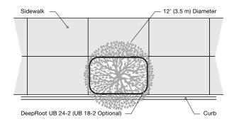
Root Pruning Applications: Root pruning can help prevent injury and preserve existing trees that are causing hardscape damage. Disruptive roots are cleanly cut and removed; linear Root Barrier is then installed. There are limitations to root pruning and a qualified Certified Arborist should be consulted.
