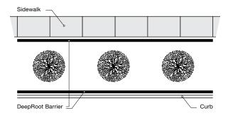
Surround Applications: Protect hardscapes that surround a planting on all four sides. Plan to line the perimeter of the planting area with the panels—this provides the maximum available uncompacted soil volume for immediate root growth.
