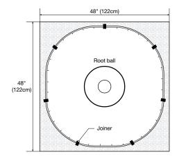
Seven (7) panels of DeepRoot UB 18-2 or UB 24-2 with a circumference of 151" (383.5 cm) fit into the square hole to form an oval.
