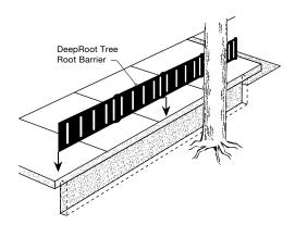
Specialty Applications: Help protect sites with unusual requirements—like tennis courts, slopes, cemeteries and retaining walls—from root damage. DeepRoot Tree Root Guides of different sizes can be used in combination in areas of variable depth.
